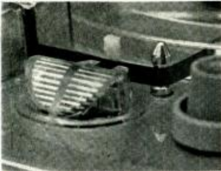
One of the unusual features is the automatic shutoff. The tape is threaded through the switch as shown. Should it break, or the end of the tape run through, the plastic finger falls forward and shuts off the machine. The switch also includes the ready and record indicators.
