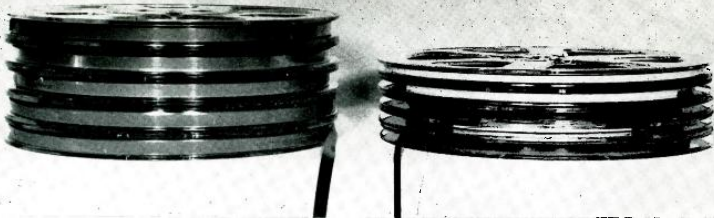
Narrow tape that can be edited without waste also saves storage space and postage on voice letters. Five reels in each stack. Demi-tape is on the right.
