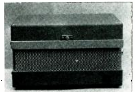
The recorder in closed position. A snap lock holds the removable lid and reels may be left on the machine with the lid closed.
