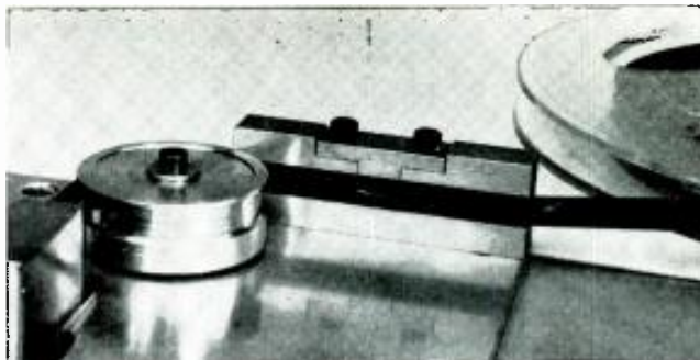
Slitting tape on the recorder can be done before or after recording. If full track recordings are slit the result will be an "original" and a "carbon."
