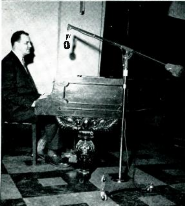
Above, a desk attachment that will attach to a conventional mike stand to provide support for a speaker's notes. It also features dual mikes, especially useful to maintain the proper sound level when a speaker turns from side to side. The mikes are Electro-Voice Mercury Model. Lower, a boom mike stand must be used on a vocalist-piano pickup to keep the stand out of the way of the player's hands.
