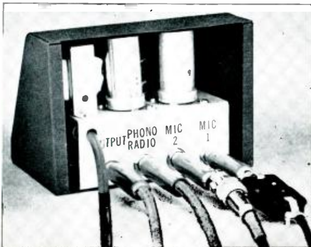
Rear view of the electronic mixer showing the output and inputs. The cable adaptors shown were rigged to fit the author's recorder. The completed unit is small and very compact so that it takes up little room:
