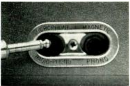
Dual outputs are a feature. An external speaker connected in one jack will operate along with the recorder's speakers. In the other jack, it cuts out the recorder speakers. A meter may also be connected to the jack for precision monitoring of recording volume. The No. 1 jack is also controlled by the monitor switch for optional operation during recording.
